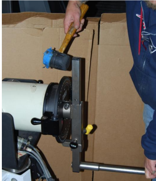
Figure 2 Removing the Input Adapter
