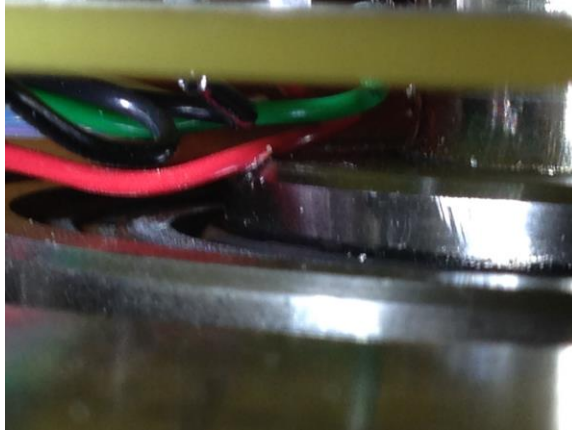
Figure 6 Stator Wire Contacting Motor Bearing
